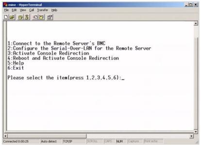
The SOL Proxy main menu allows you to change the SOL settings of a remote managed system's BMC, reboot the remote BMC, or activate console redirection.
